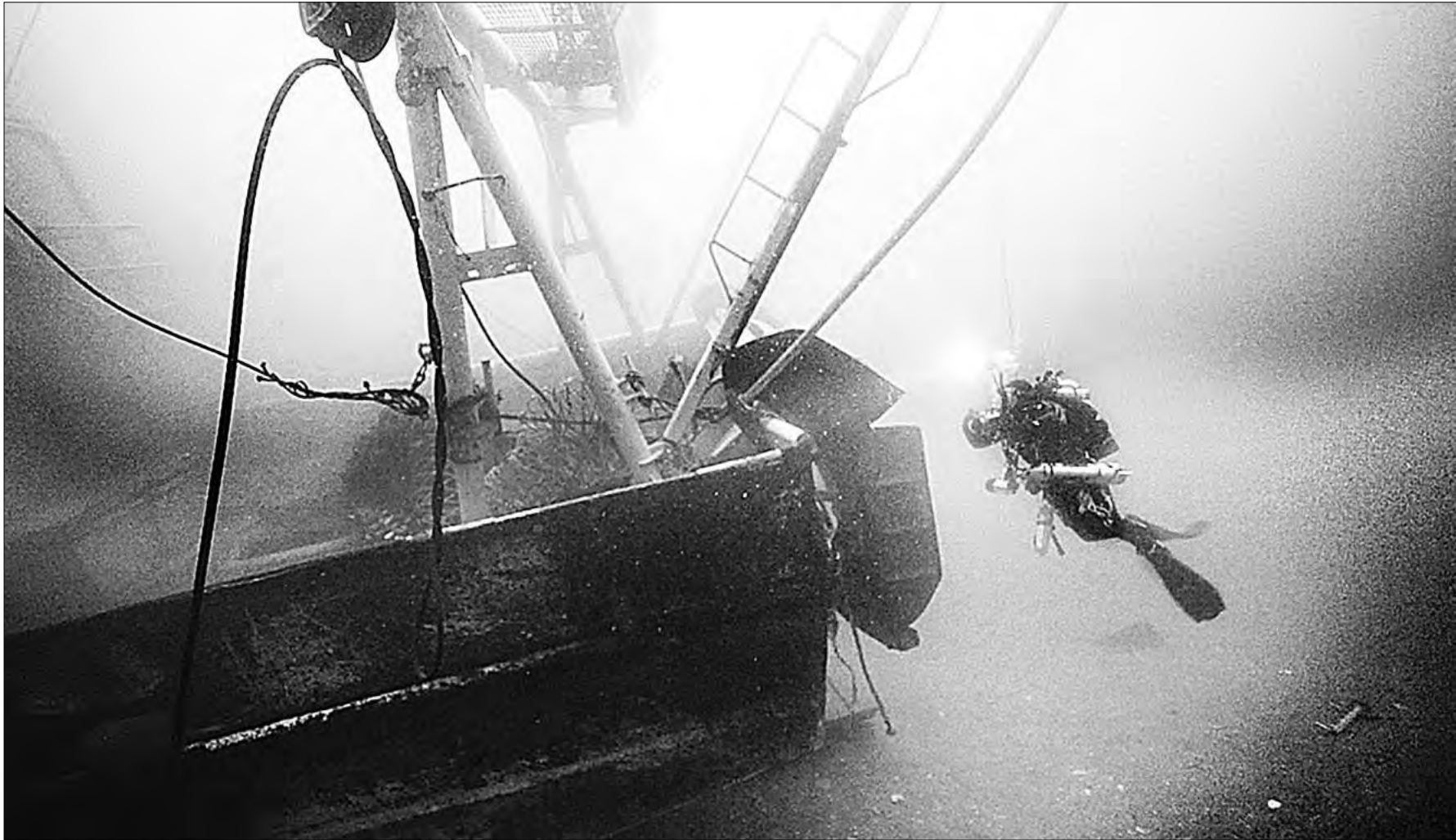
Gatto looks over the heavily damaged stern of the Lady Mary. None of the divers on the scene said they had seen this kind of destruction, despite having explored hundreds of wrecks. Experts who believe the fishing boat was struck by a large commercial ship point to this severe, localized damage. Bradley Sheard
